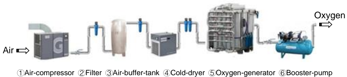
Figure2. Structure Compose and the principle of the COSS
